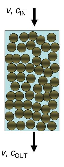
Natural Packed Bed – subsurface with groundwater flow
